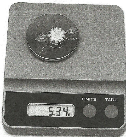
Figure 6 This laboratory scale measures to the nearest hundredth of a gram.
