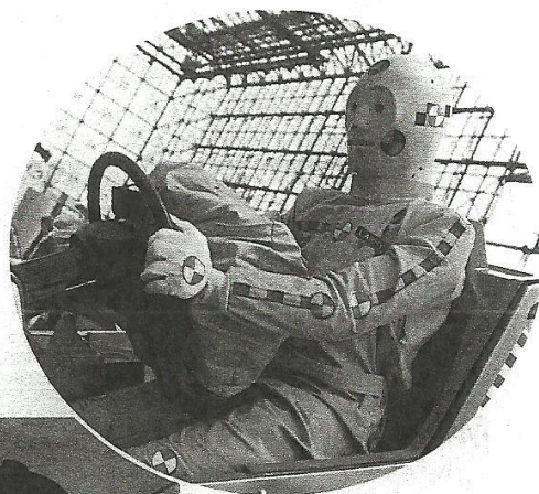
Crash-test dummies are used to test vehicles without putting people in danger.
