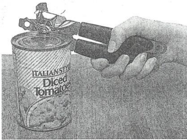
Figure 16 The can opener changes the small force of your hand on the handles to a large force on the blade that cuts into the can.
